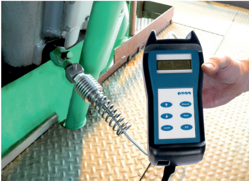
EPM-XG in operation on a gas compressor
